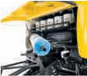
Integrated prop to support a roll of net when changing it from ground level.
