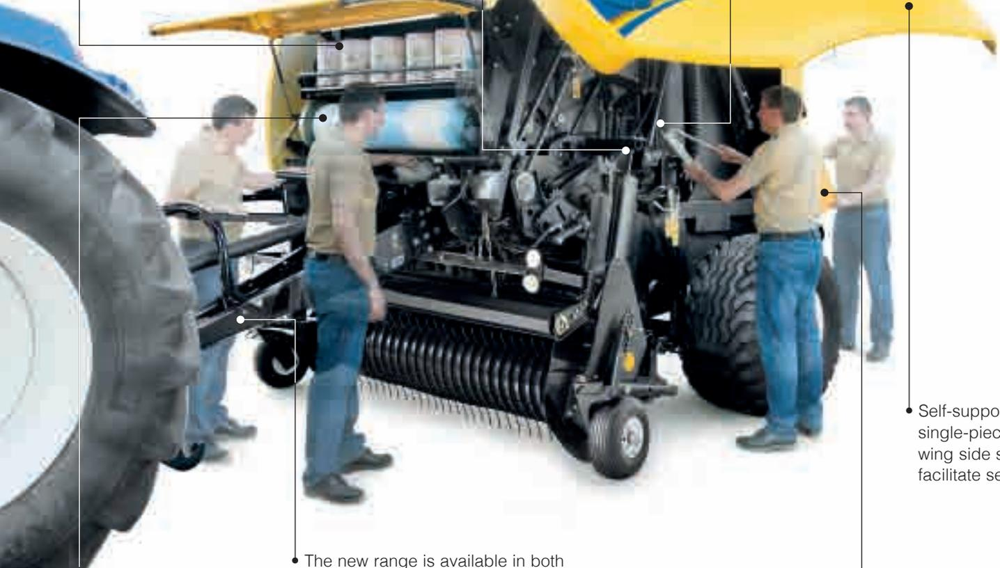
Self-supporting, single-piece gull wing side shields facilitate servicing.
